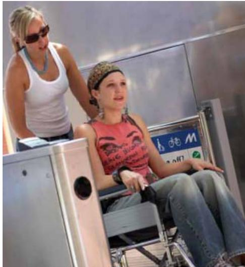
**SmartRider fare gates accommodate wheelchairs, with SmartRider card processor mounted on side**
